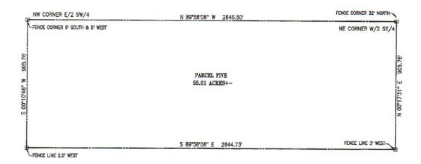
THIS PLAT OF SURVEY MEETS THE OKLAHOMA MINIMUM STANDARDS FOR THE PRACTICE OF LAND SURVEYING AS ADOPTED BY THE OKLAHOM STATE BOARD OF REGISTRATION FOR PROFESSIONAL ENGINEERS AND LAND SURVEYORS.
